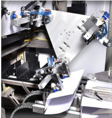
*Planetary rotary motion placer (zero velocity at pick up and placement). Level of degree is 120 degree or 240 degree with vacuum pre-brake.*
