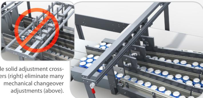
Single solid adjustment cross-members (right) eliminate many mechanical changeover adjustments (above).
