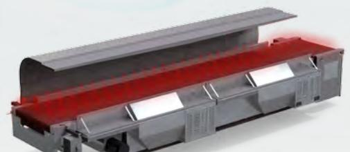
**Evenly heated air** passing through the conveyor web contacts the film under the product resulting in consistent "air weld" of the film lap seam. Tunnel chain temperature and airflow are precisely adjusted through product specific recipe-driven changeovers. Poor lap sealing or holes melted in the seams are eliminated, resulting in strong and even seams that hold up to the rigors of distribution and stocking operations.
