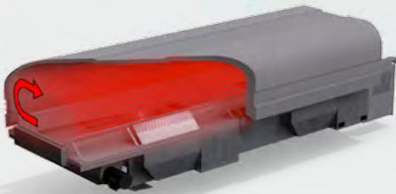
The **heat system** is designed so the air supplied to the distribution system is perfectly uniform, eliminating film distortion due to hot or cold pockets. The Contour continuously recycles the air as it heats, decreasing the amount of energy required to reach operating temperature. A well insulated heat tunnel minimizes heat loss, which also maintains a safe outer surface temperature.
