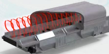
At the **heart** of this innovation is a unique combination of design features which result in "laminar" airflow, rather than "turbulent" airflow, which most shrink systems use today. Unlike turbulent airflow, which causes a multitude of shrinking inconsistencies, our proprietary laminar design precisely balances the heated air, perfectly "coating" the film from every direction, shrinking and sealing the film in an even, predictable manner.
