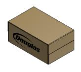
REGULAR SLOTTED CASE (RSC) END LOAD MFG FLAP ON SIDE PANEL
