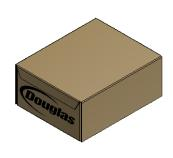
FULLY OVERLAPPED (FOL) SIDE LOAD MFG FLAP ON TOP PANEL
