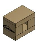
REGULAR SLOTTED CASE (RSC) WITH REVERSE FLAP FOLDING
