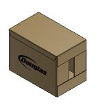
REGULAR SLOTTED CASE (RSC) WITH REVERSE FLAP FOLDING
