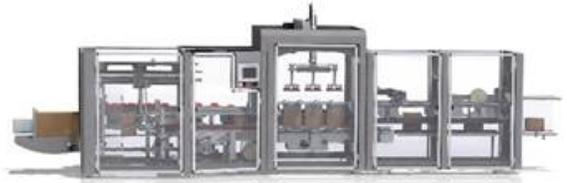
**Axiom® IM** – Case packing up to 40 cases/min with precise product control, capable of packing in wraparound or knockdown style cases and trays, with or without partitions.
