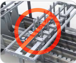
Single solid adjustment cross-members (right) eliminate many mechanical changeover adjustments (above).
