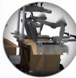
Timing and motion of case squaring and compression for sealing the case.
