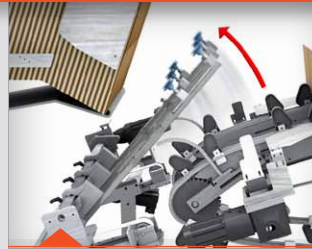
corrugated pick arm motion (Axiom ARC pictured)
