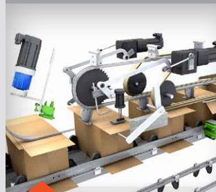
case squaring and compression for sealing case
