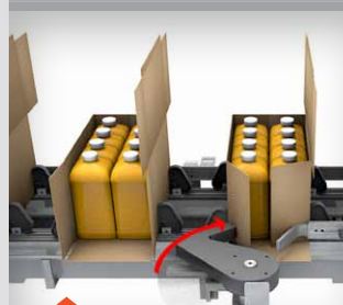
flap tucker timing and motion
