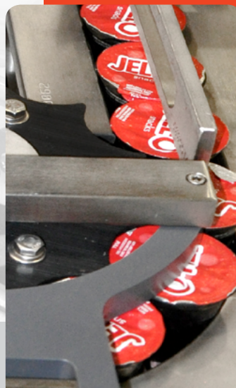
◀ Star wheels for soft products requiring surge control and spacing
